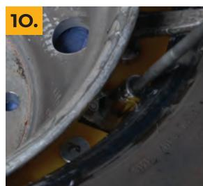
10. With a tire iron, pry the tire away from the rim to expose the gearbox and tighten gearbox with ratchet and extension making sure both Retroband halves close fully
