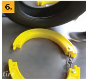
6. With one half of the Retroband assembled with one gearbox we now install both halves of the Retroband into the tire
