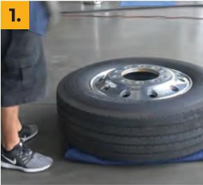
1. Remove tire and wheel assembly and lay face up
