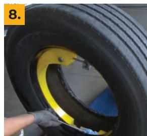
8. Lubricate both inner and outer bead of the tire, inside the rim and the inside of the Retroband
