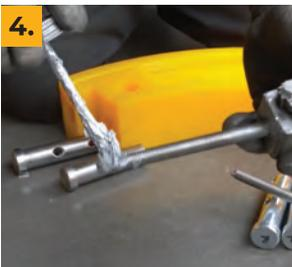
4. Assemble two Retroband halves with one gearbox and two pins, one right hand threaded pin and one left hand threaded pin
