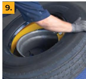
9. With the rim face down install the tire and Retroband assembly over the rim
