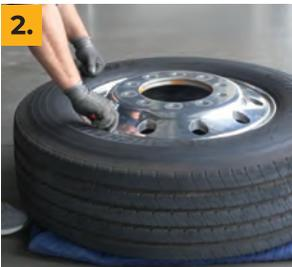
2. Remove valve core and deflate the tire
