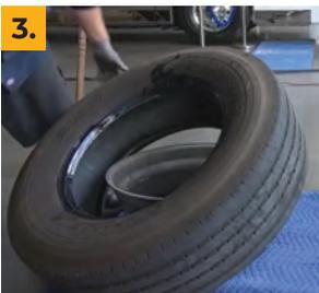
3. Break bead of tire and remove tire from the wheel
